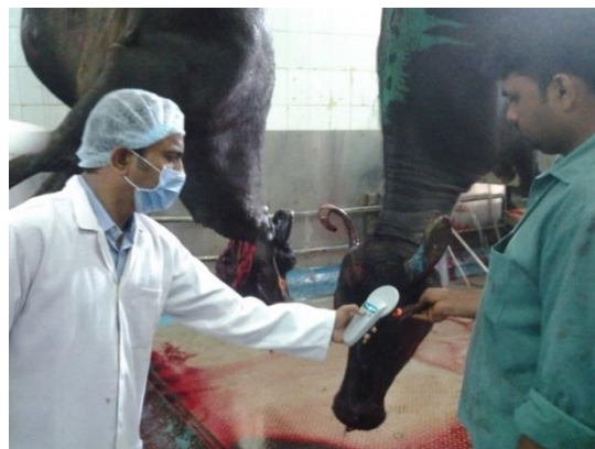
Fig 4: Reading of tags using RFID reader in the slaughter line
